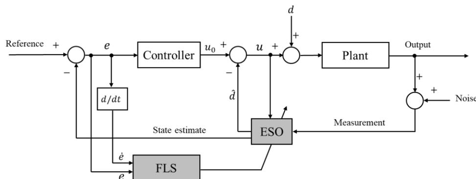
Figure 1. Block diagram of control loop with fuzzy logic system (FLS)-based extended state observer (ESO)
